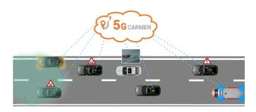
Fig. 1. Back-situation awareness in 5G-CARMEN. The ambulance in the bottom, right-hand side corner of the figure exploits the 5G framework, consisting of C-V2X communication and MEC, to inform the other vehicles about its ETA, so that the lane can be proactively cleared.
